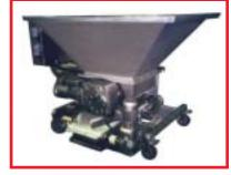
Showing with hopper, frame and conveyor.
